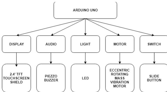
Fig. 3. Decomposition of Hardware Modules
