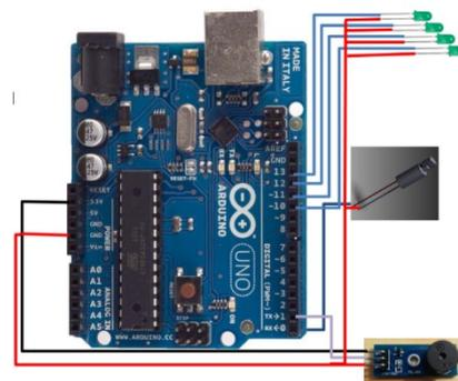
Fig. 5. Alarm System, LED, and Compartment Indicator Components
