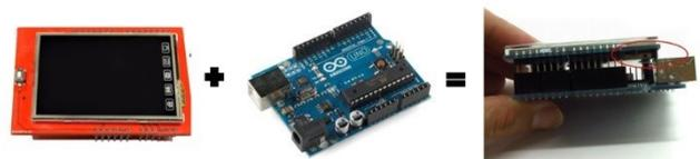
Fig. 4. Arduino and 2.4 TFT Touchscreen Shield
